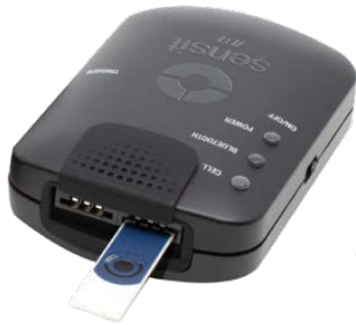
Sensit BT.SPE with screen printed electrode
