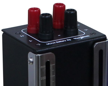
banana socket panel & height ruler
