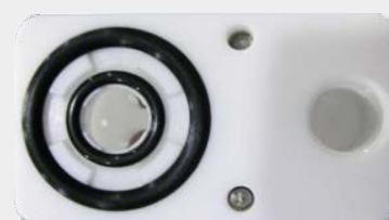
Active area will be determined by O-ring's position.
