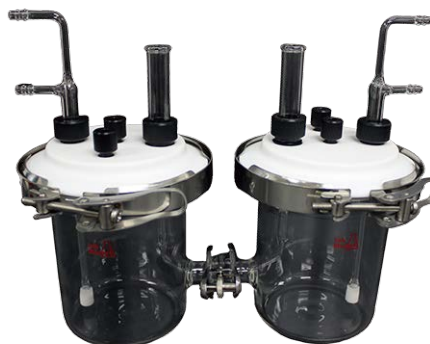
HCELL1 H-Type Cell with optional flag type Pt counter electrode
