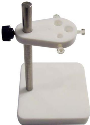
The universal electrode holder, UEH1, is designed to hold various sizes of electrode. The UEH1 has 4 holes to hold electrodes and three of them have a screw to adjust its hole size. The hole size is available from 1.6mm to 10mm. The material of plate is Teflon®, which has high resistance to chemicals and its white color helps user to recognize a tiny change of samples during experiments.
