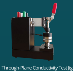
Through-Plane Conductivity Test Jig
