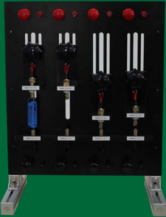
High current Universal Battery Jig 4PK-UCJH4-4P
