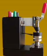
Through-Plane Conductivity Test Jig
