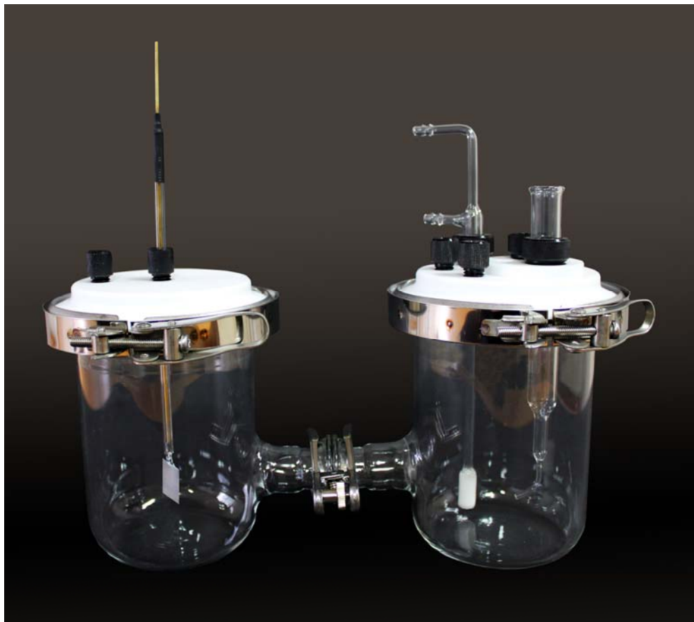
HCELL1 with optional Pt plate counter electrode
