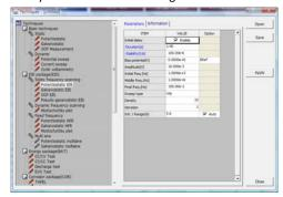
4. Select Potentiostatic EIS at left technique selection region. The parameter editing region is located at right. Input figure for parameter setting as the follows.
