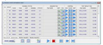
To start experiment for specific channel, click Start button on the channel. If you want to start experiment for multiple channel, click on Group column which you want to start and click Start button at bottom side.
