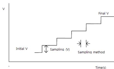
This function is for high capacitive sample such as supercapacitor, corrosion, battery etc.
