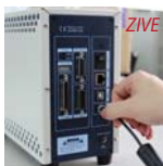
Plug in the potentiostat's power cord.
