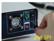
Plug in the potentiostat's power cord.
